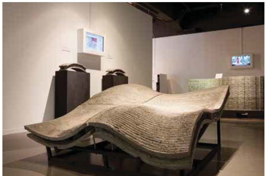
Figure 4. Doubly curved surface fabricated by the Freeform Construction team, Loughborough University. Photo: Dr. Richard Buswell and Professor Simon Austin, Loughborough University.
