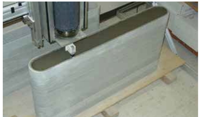
Figures 1 and 2. Contour Crafting “24 Hour House” and a panel prototype being fabricated. Images: Dr. Berok Khoshnevis, professor, University of Southern California.
